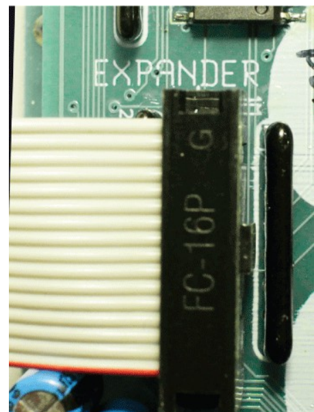
QCD Expander: all jumpers removed and ribbon cable connected to the Expander module
