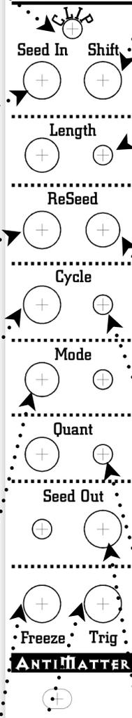
**Shift in jack:** -5 volt to +5 volt CV input that transposes the Seed Out.
