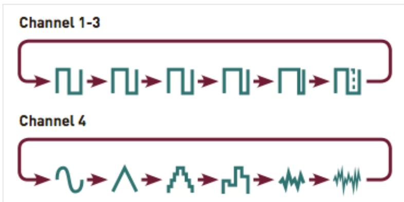
For channel 1, 2, and 3, the waveshapes are all square waves with 50%, 66%, 75%, 87%, 95% pulse or CV controlled pulse width. With this last option, channel 4's frequency input doubles as a PWM control.
