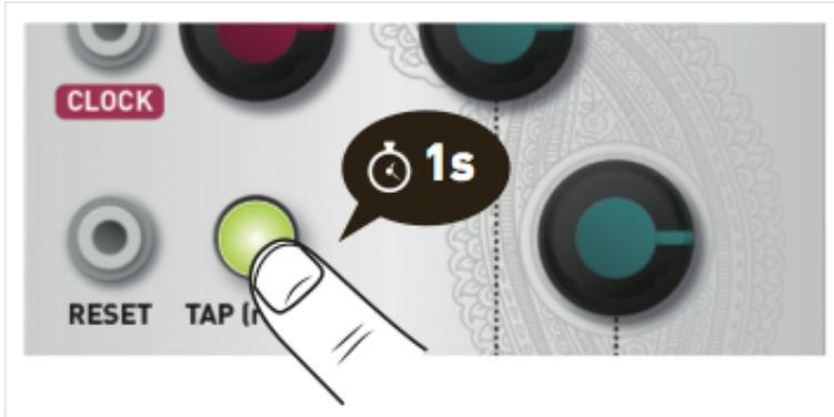
Unplug all CV inputs and hold the **TAP/reset** button for half a second to adjust Grids' options. The switch stays illuminated. Hold the button again for half a second when you are done.
