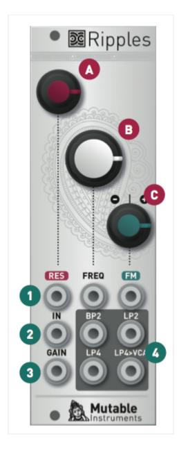
**RES**: Resonance control voltage, added to the value set by the RES knob. A control voltage of +4V starts bringing the filter to self-oscillation. Control voltages above +5V are compressed and only bring a moderate increase of the loudness of the self-oscillation tone.
